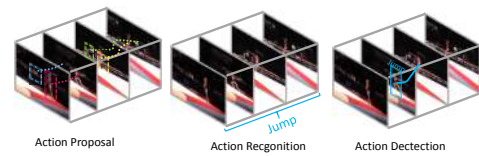
Fig. 1. Conceptual illustration of the difference among action proposal, action recognition, and action detection. Action proposal tries to extract all possible human actions which are highlighted using dash-lines. Action recognition aims to classify the whole video into specific categories, e.g., ‘Jump’. Action detection aims at detecting when and where a specific action appears (highlighted using solid-lines).
